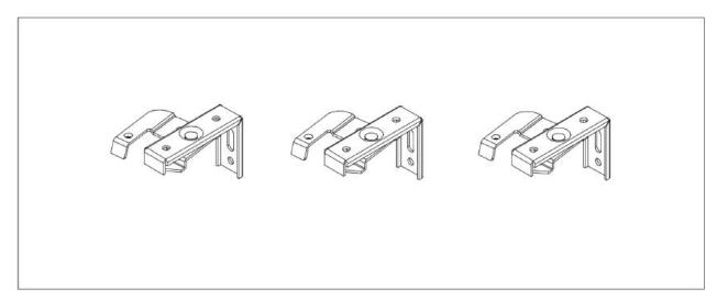
Step I Install the mounting hangers in such a way that they do not interfere with the components inside the gutter. The wooden blind must be mounted horizontally for it to work correctly.
