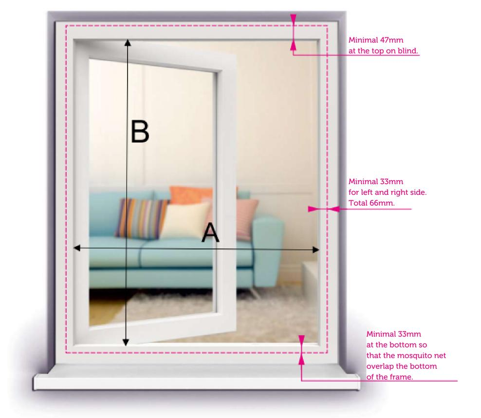
Open the window sash and measure the width of the outer window frame as shown on figure 1.
