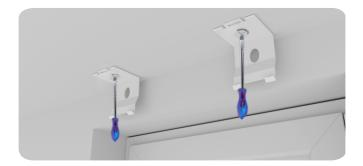
Stage IV Mount the blind in bolted mounting hangers.
