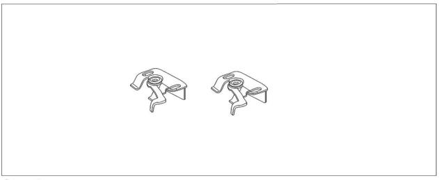
Step I Install the mounting hangers in such a way that they don't interfere with the elements inside the gutter. For the blind to work correctly it must be mounted horizontally.
