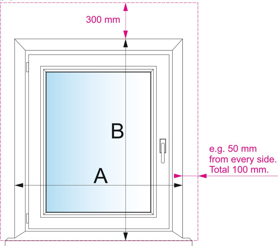
Measure the width and height of the window recess. Fig. 1.
