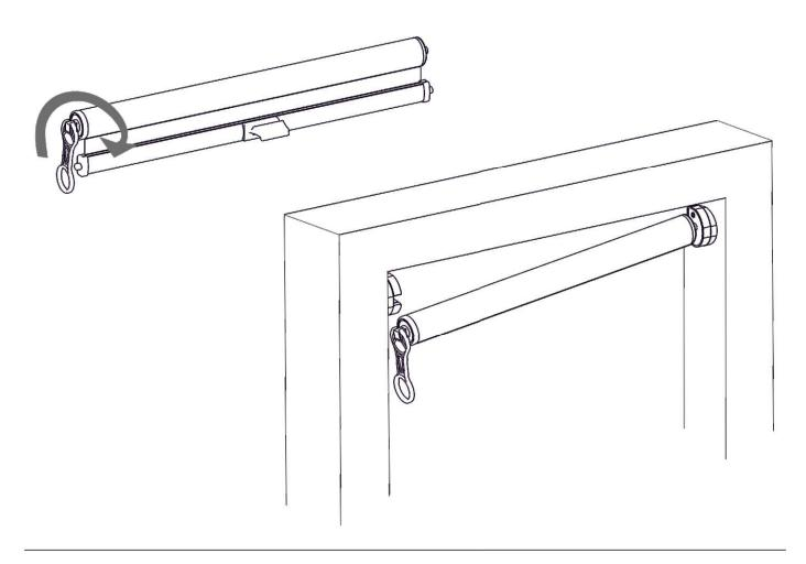
Step III After installing the blind in the holders insert the handle plug to prevent the blind from falling out.
