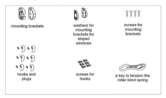
Step I Screw on the mounting brackets. If the window frame has a slant, use washers for the mounting brackets. If the window frame doesn't have a slant, do not use washers.
