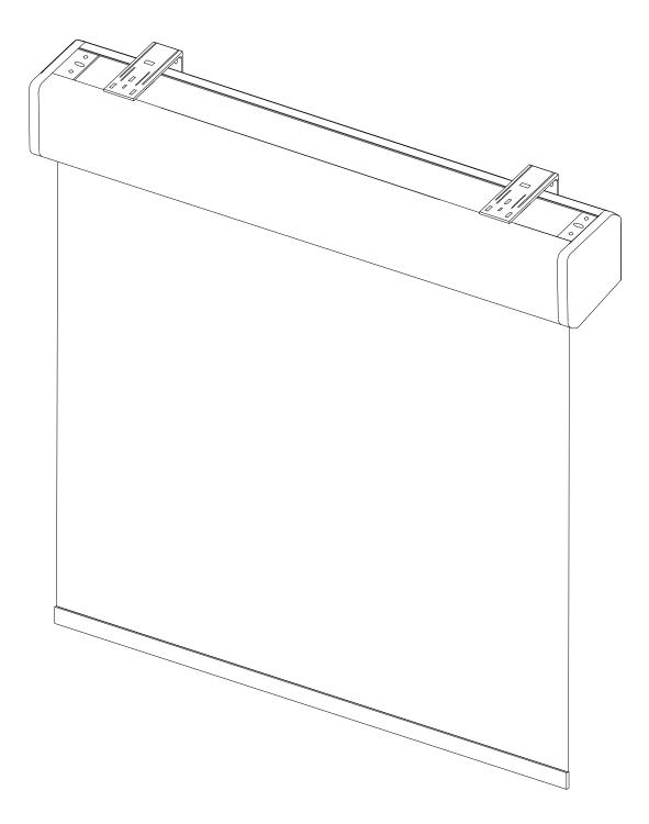
The following mounting brackets are supplied with the roller blind. Their number depends on the width of the roller blind. Minimum 2 pcs, maximum 4 pcs.
