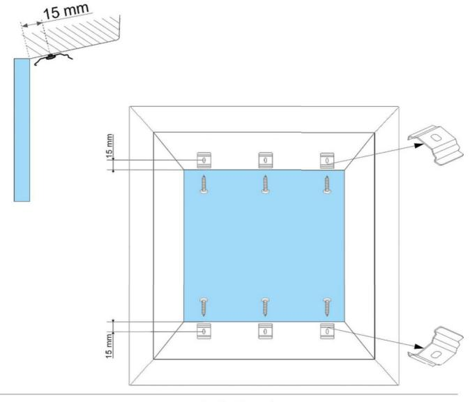
Step II In mounted clips press bottom and top profil of the pleat. Next put on the handles for operating the pleat. Below illustration explain the way of installation.
