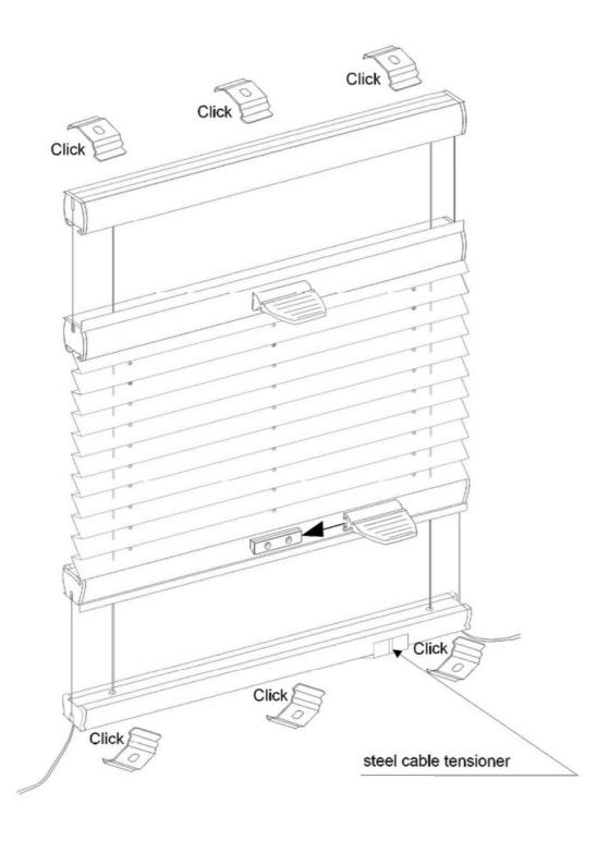
Step III Adjust the optimal tension by moving the steel cable tensioner left or right. This line prevents the fabric from hanging.
