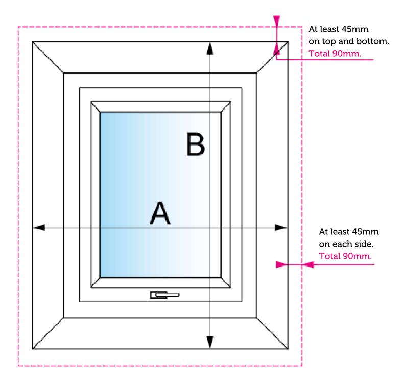
Measure the width and height of the window recess (hole in the wall). Figure 1.
