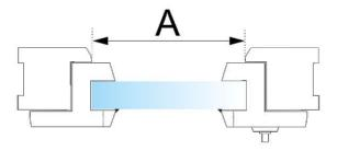
The overall size of the mosquito net will be 24 mm wider and 24 mm higher than the given measurement A and B.
