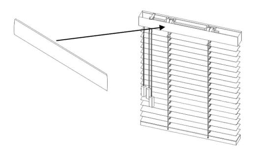
If a masking cover with sides has been selected, attach it using the supplied angle brackets.
